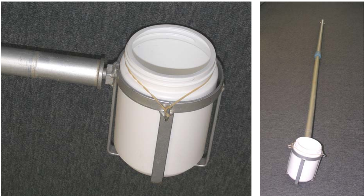
Figure 1. Sampling pole used to collect pond effluent samples.
